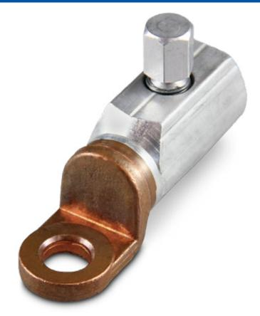
VCXI lugs consist of an aluminium barrel linked to a copper palm by friction welding technology. The aluminium barrel is provided with a shear head bolt controlling the tightening torque.
